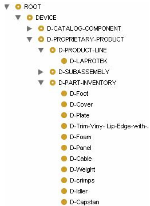
Figure 8. Part of the device taxonomy for the surgical robot design
