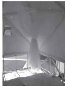
Frameless hard-panel structures of precision diecut panels made from flame-retardant UVresistant corrugated polypropylene, configurable as needed. The initial TranShel exemplifies a design paradigm that can achieve diverse shelters appropriate for different climates and cultures.
