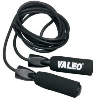
Figure 4: The Valeo jump rope. 5 Made from rubber, the jump rope had slight springback and tight packaging caused some bends along the length of the rope. The rubber rope stretched some, but for all analysis, this minor extension and the springback are neglected.
