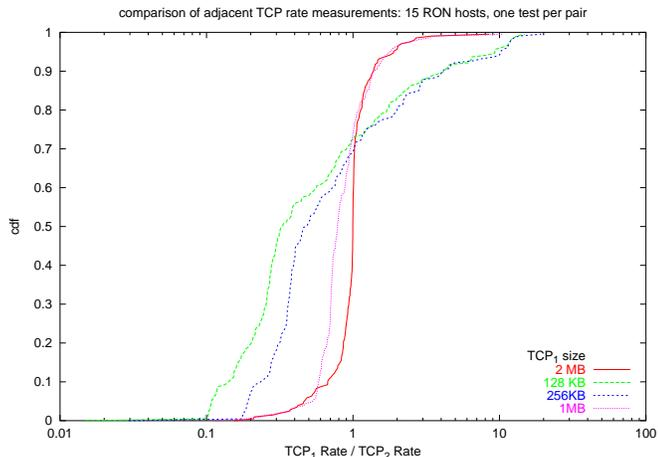
Fig. 3. Ratio of throughput achieved by first tcp transfer to second tcp transfer
