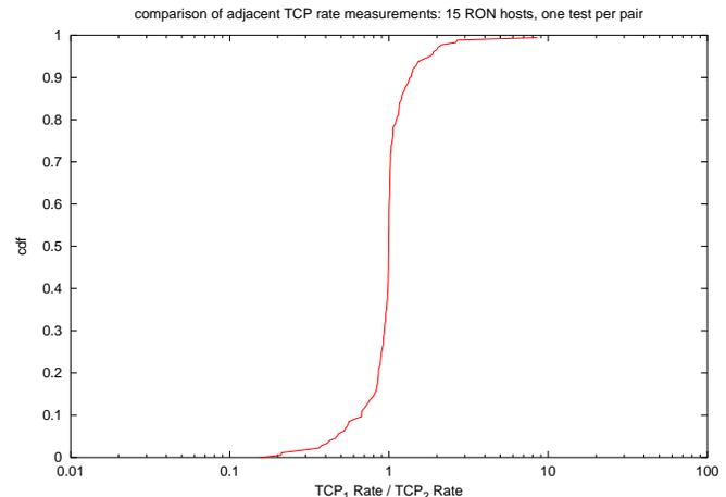
Fig. 1. Ratio of throughput achieved by first tcp transfer to second tcp transfer
