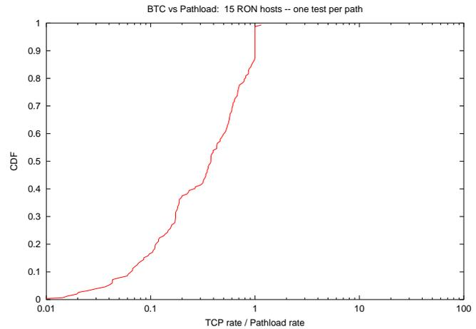
Fig. 2. Available Bandwidth as measured by Pathload, vs. BTC as measured by TCP rate. The Pathload rate is a range – the closer of the range endpoints for each point is used. If the TCP rate falls within the range, a ratio of 1 is plotted.
