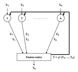
Fig. 3. An architecture with more feedback.
