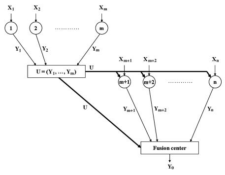
Fig. 2. The daisy chain architecture.
