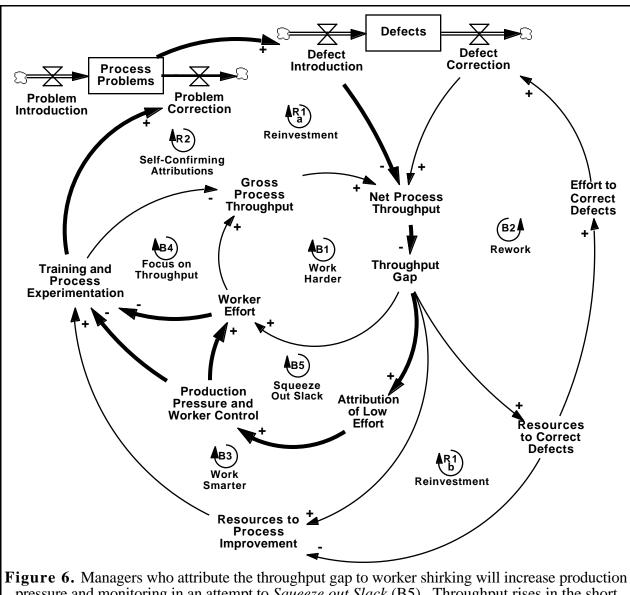
**Figure 6.** Managers who attribute the throughput gap to worker shirking will increase production pressure and monitoring in an attempt to *Squeeze out Slack* (B5). Throughput rises in the short run, but production pressure pulls resources away from improvement activity, leading to erosion of process capability and still lower throughput (reinforcing loop R2).
