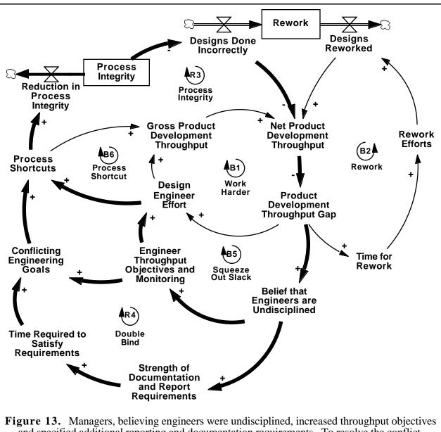
and specified additional reporting and documentation requirements. To resolve the conflict, engineers cut corners, reducing the integrity of the process, leading to still more defects and still lower productivity. Management's belief that engineers were undisciplined was reinforced.
