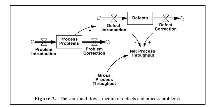
Figure two represents *Defects* and *Process Problems* as stocks (level or state variables) denoted by rectangles (Forrester 1961). A stock is the integration (accumulation) of its inflows less its outflows, denoted by the straight arrows with valves. For example, the defect stock accumulates the rate of defect introduction less the rate of defect correction:
