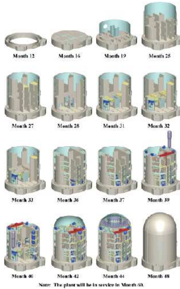
Figure A.8: ACR-700 construction sequence for first unit (Source: [40])
