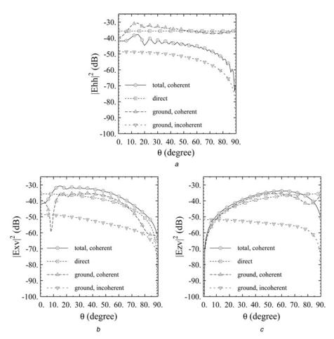
**Fig. 8** Components of the received power as a function of the transmitter height for a fixed distance (20 $\lambda$ ) between the transmitter and receiver The observation point is at (0, 0, 0.2 $\lambda$ ), and the source is at (20 $\lambda$  sin $\theta$ , 0, 0.2 $\lambda$  + 20 $\lambda$  cos $\theta$ ) at  $Q = P = \hat{h} = \hat{y}$  b and  $Q = P = \hat{v} = (-\sin\theta, 0, \cos\theta)$ ,  $Q = \hat{v} = (-\sin\theta, 0, \cos\theta)$
