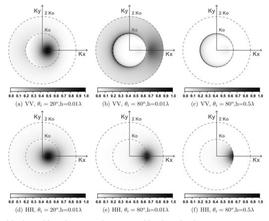
**Fig. 4** Spectral distribution of the incoherent scattered power generated from the rough surface a and d For vv- and hh-polarisation, respectively, at the incidence angle  $20^{\circ}$ , and the height is  $0.01\lambda$  b and e For vv- and hh-polarisation, respectively, at the incidence angle  $80^{\circ}$ , and the height is  $0.01\lambda$  c and f Same as (b) and (e), but the height is  $0.5\lambda$
