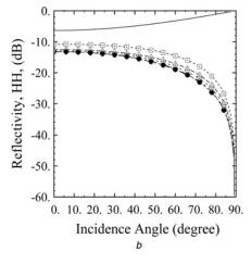
Fig. 3 Comparison between the coherent and incoherent reflectivities against incidence angle
