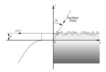
**Fig. 1** *Inhomogeneous half-space medium with a rough interface* Left side of this figure shows the dielectric profile
