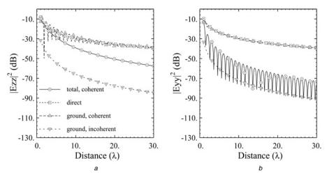
**Fig. 6** Electric field against the distance between the source and observation point The underlying ground is homogeneous ( $\varepsilon = 8 + i1$ ). The rough surface has an exponential correlation function, ks = 0.3, and kl = 3.0 a  $\mathbf{Q} = \mathbf{P} = \hat{z}$  b  $\mathbf{Q} = \mathbf{P} = \hat{y}$
