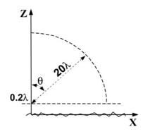
**Fig. 7** Distance between the source and observation point is fixed at  $20\lambda$ , but the source point is moved on a circle of radius  $20\lambda$  in the x-z plane
