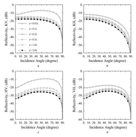
Cross-polarised incoherent scattered fields against incidence angle
