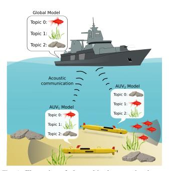
Fig. 1: **Illustration of the multi-robot terrain characterization problem**. Each individual AUV builds its own local topic model. Model parameters from all vehicles are transmitted top-side via acoustic modem, where the models must be combined into a consistent global model. However, there is no guarantee that the individual robots will agree on which visual category corresponds to each topic ID. This correspondence issue must be addressed to achieve global consensus.
