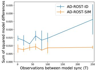
Fig. 5: Sum of squared differences in topic-word distributions on each model evaluated on the *first* mission. As we increase the number of observations between model synchronization steps, the topic distributions begin to diverge in the case of AD-ROST-ID. AD-ROST-SIM is comparatively robust to decreases in communication rate.
