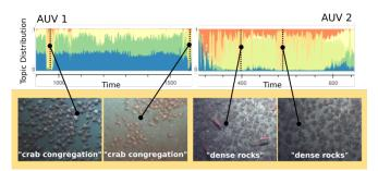
(a) Topic distributions predicted by AUV 1 and AUV 2 using the AD-ROST-ID method. AD-ROST-ID results in *different* visual categories being assigned to the same topic.
