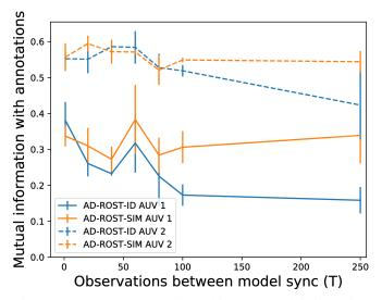
Fig. 4: AD-ROST-SIM achieves higher mutual information than AD-ROST-ID as we increase the period between model synchronizations. Despite requiring a fraction of the data transmission, the mutual information of AD-ROST-SIM with T = 250 is comparable to that of either method with T = 1.
