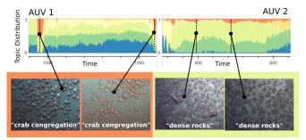
(b) Topic distributions predicted by AUV 1 and AUV 2 using the AD-ROST-SIM method. Matching by topic similarity helps to ensure that distinct visual categories are appropriately assigned to different topics.
