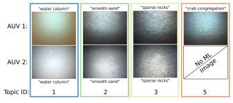
(b) Exemplars from the model inferred using AD-ROST-SIM with T = 100 show that the model successfully assigns different topics to different visual categories. Additionally, when a particular category is observed by one AUV but not the other, such as in the case of the "crab congregation," there is no image from AUV 2 where the corresponding topic occurs with maximum likelihood.
