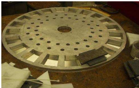
(a) PM Rotor: The slots where the magnets go in are clearly visible. A sample magnet is also shown.
