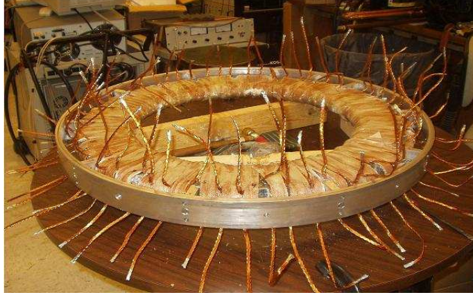
Figure 2.4: Stator: The winding ends here are yet to be soldered before the stator is assembled with the rest of the machine.
