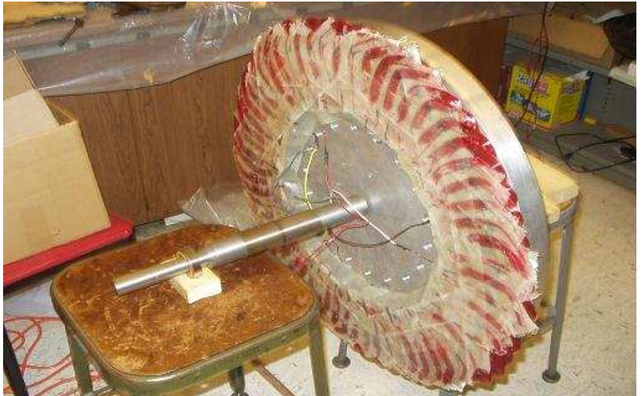
Figure A.1: Wound power rotor fabricated of 120 coils using standard 16 AWG wire and finished with epoxy and glass cloth wrap. the aluminum plate on which the arrangement is mounted is slotted for ventilation and has a keyed hole at the center. This component has a mirror component similar in every aspect. After fabrication the rotor was balanced using a ‘static balance’ technique; adding/removing material from the outside face just inside of the outer periphery by drilling holes (removing weight) or screwing bolts (adding weight).
