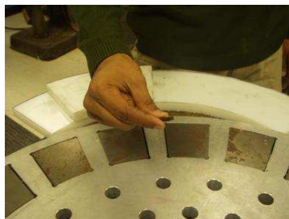
(c) PM Rotor: Poling the magnets to ensure that they are placed correctly in the N-S-N-S fashion.
