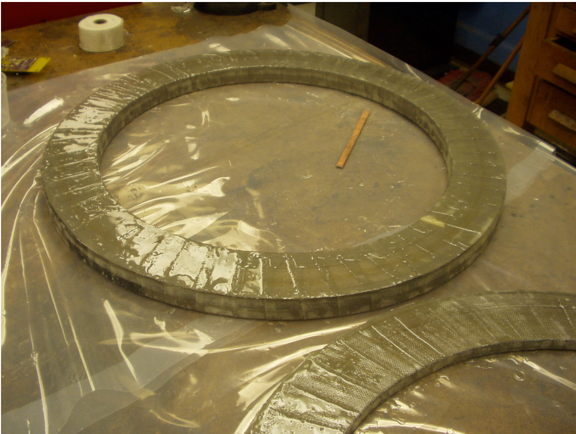
Figure B-1: Completed Stator Core
