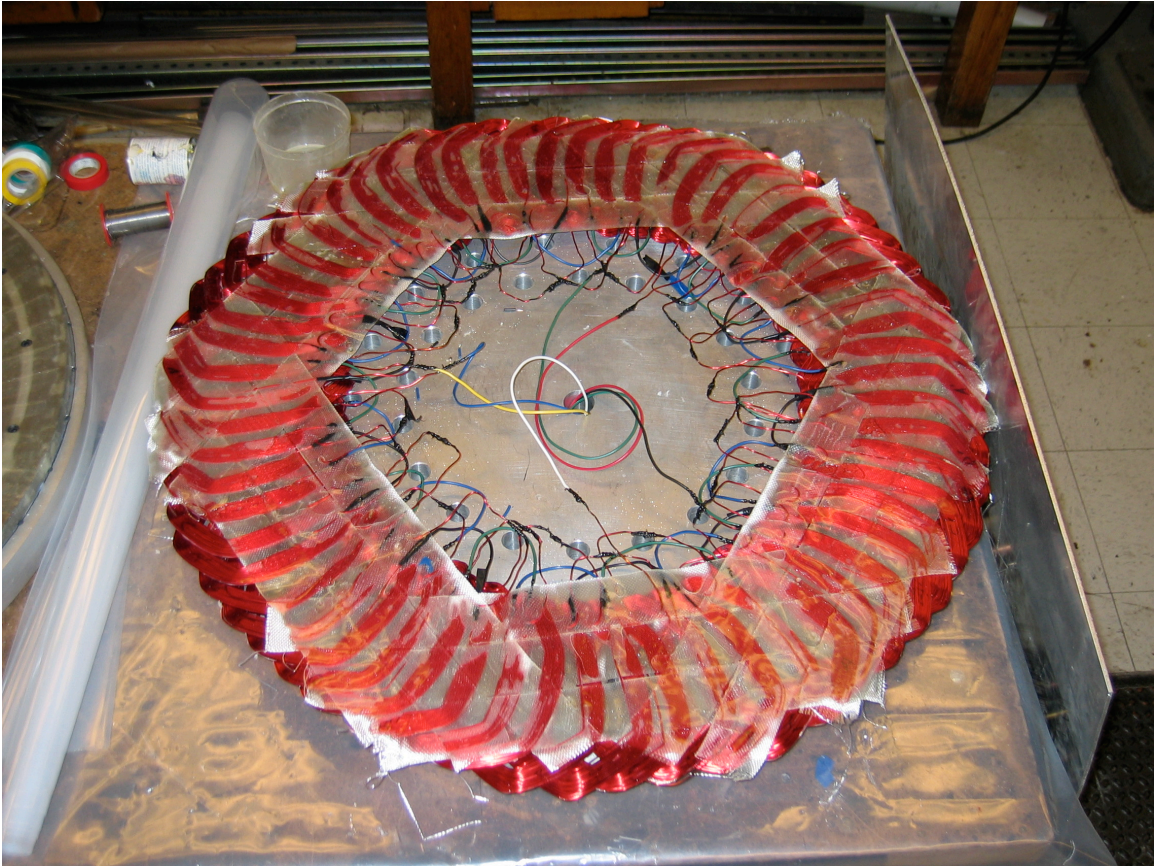
Figure B-5: Power Rotor with Windings
