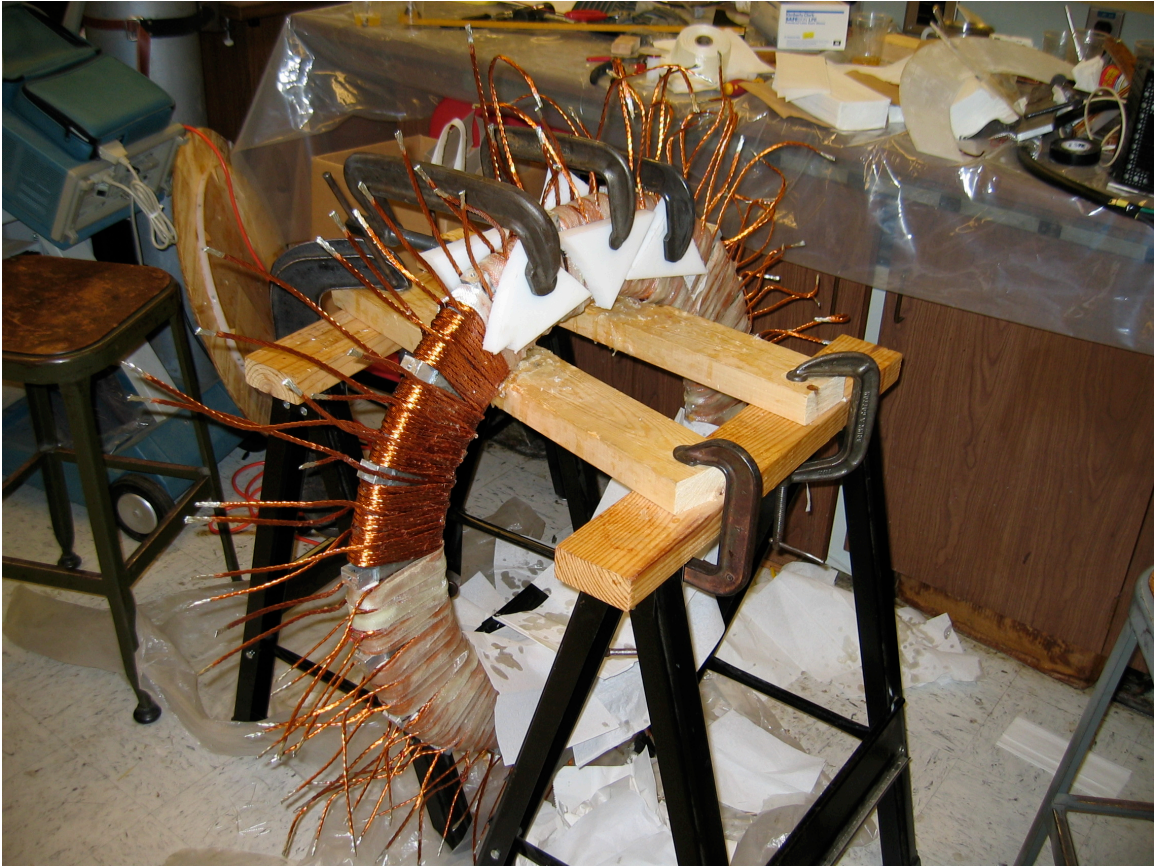
Figure B-3: Wound and Partially Fiberglassed Stator
