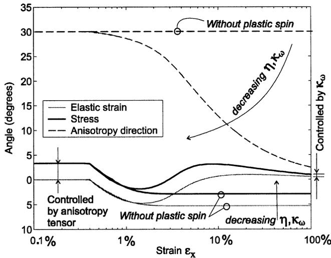
Fig. 1. Rotation of the principal directions of elastic strain, stress and of the anisotropy tensor with initial value  ${}^0 \mathbf{P}_1 = [\cos 30, \sin 30, 0]_X^T$ .
