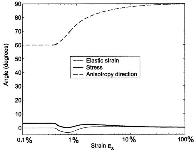
Fig. 2. Rotation of the principal directions of elastic strain, stress and of the anisotropy tensor with initial value  ${}^0\mathbf{P}_1 = [\cos 60, \sin 60, 0]_X^T$ .
