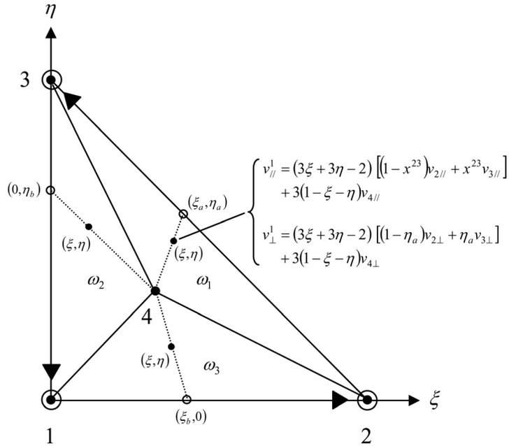
Fig. 2. Illustration of the interpolation of velocity  $\mathbf{v}$  (see [8]).
