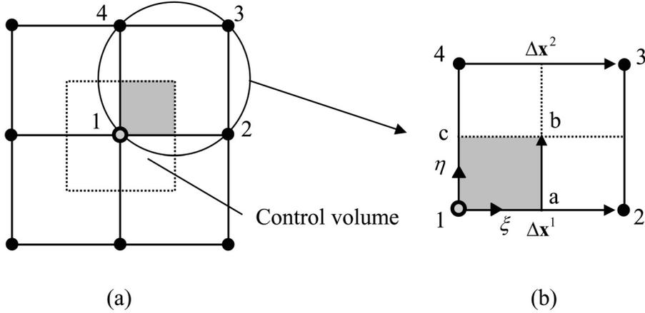
Fig. 1. Control volume on the four-node element: (a) four-node element; (b) section ab.
