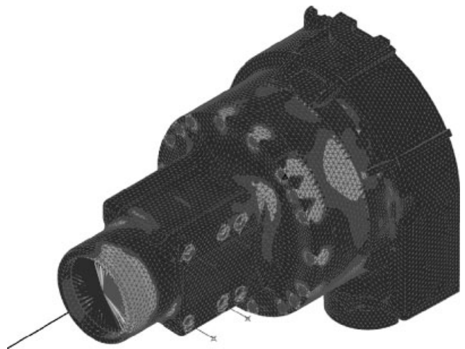
Figure 5. Model of a rear axle; about a quarter of a million elements, including contact solved in about 20 minutes on a single-processor PC.
