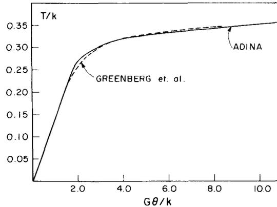
Figure 2. Elastic-plastic analysis of torsion problem ( $k = 100/\sqrt{3}$ ,  $\theta =$  rotation per unit length)
