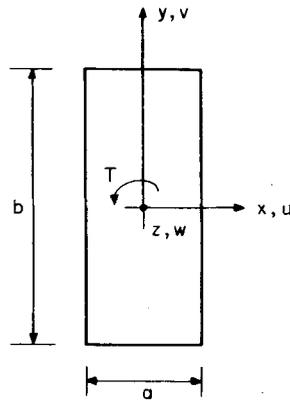
Figure 1. Rectangular section subjected to torque  $T$  resulting in rotation per unit length  $\theta$
