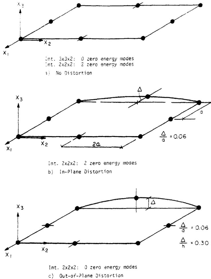
Fig. 10. Spurious zero energy modes in 8-node shell element.
