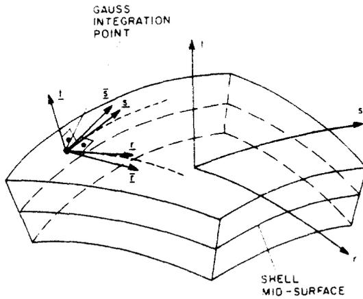
$$\bar{i} = \frac{s \times t}{|s \times t|} \quad ; \quad \bar{j} = \frac{t \times \bar{i}}{|t \times \bar{i}|}$$
