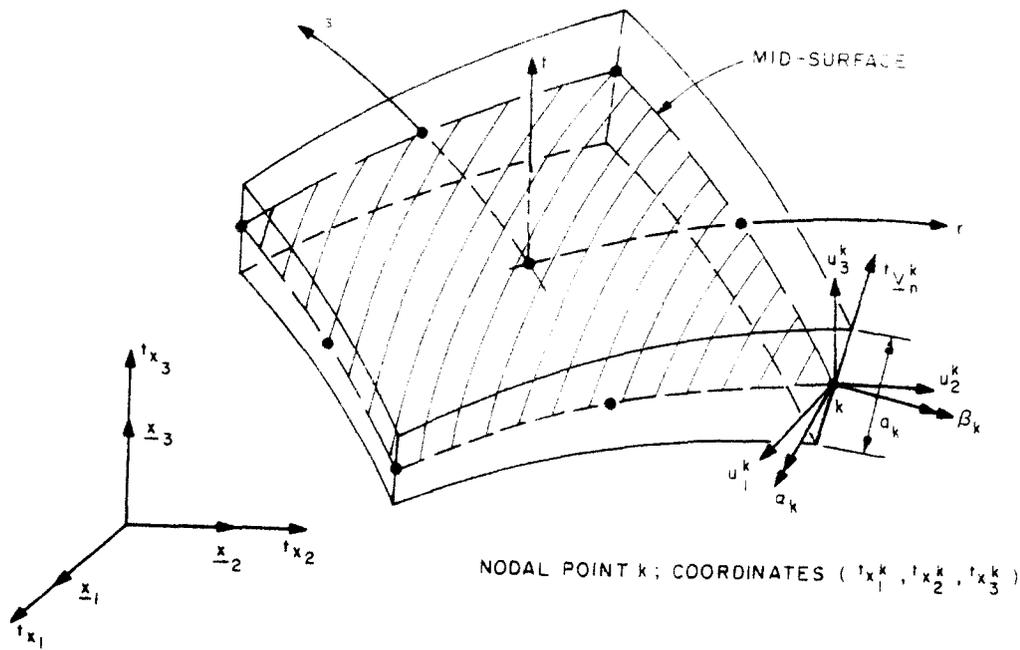
Fig. 1. Isoparametric (degenerate) nine-node shell element.
