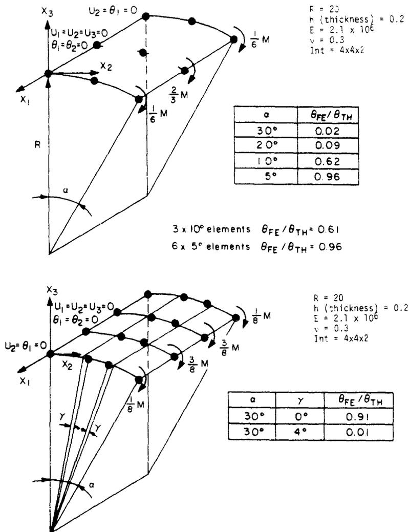
Fig. 9. Analysis of curved cantilever model. Note that the integration order for the parabolic element is higher than used in practice, and that at  $\gamma = 4^\circ$  the cubic element is highly distorted (not shown to scale).
