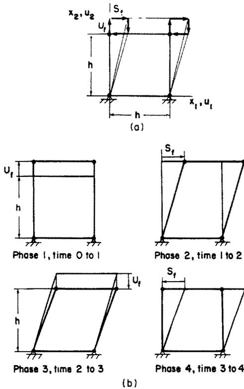
Fig. 1. Problem analyzed. (a) Strain path considered. (b) Individual strain phases.
