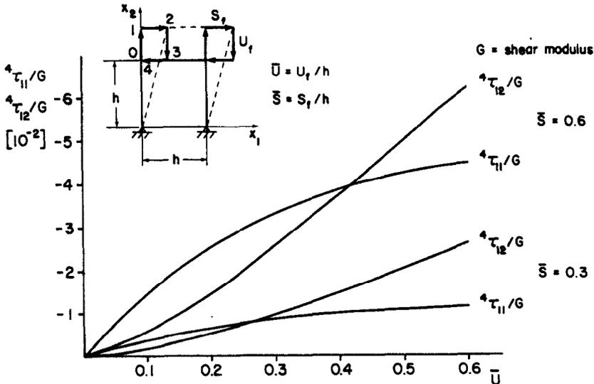
Fig. 2. Residual stresses as functions of elongation and shear measures  $\bar{U}$  and  $\bar{S}$  (U.L.J. analytical solution).
