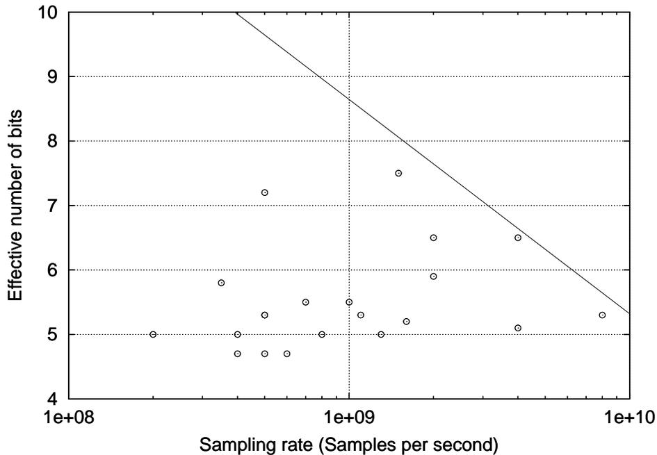
Figure 5: All high-speed flash A/D converters: effective number of bits versus sampling rate. The line corresponds to the limitation imposed by an rms aperture jitter of 0.4 ps.
