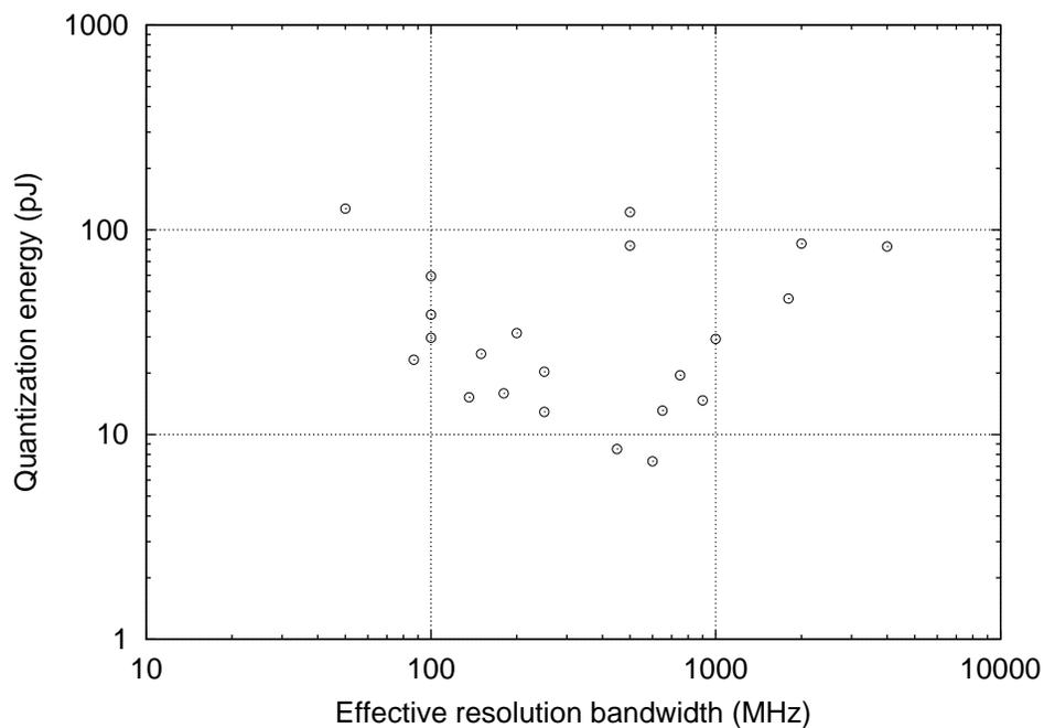
Figure 3: All high-speed flash A/D converters: quantization energy versus effective resolution bandwidth.
