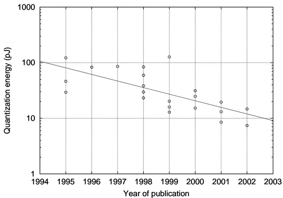
Figure 4: All high-speed flash A/D converters: quantization energy versus year of publication. The best-fit line shows a factor of ten improvement in quantization energy over nine years.
