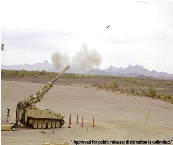
**BAE is building the NLOS-C is a 23-ton, 155mm, high-caliber, self-propelled cannon system developed for the U.S. Army under the Future Combat System (FCS). The system includes a Breach Mount Laser Ignition System (BMLIS) fire control that provides for the automated high repetition rate firing of munitions from remote locations.**
