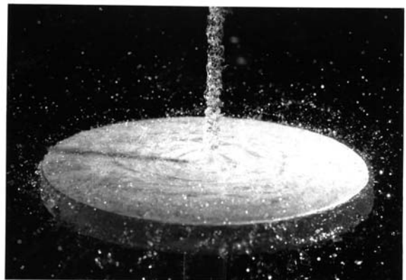
Figure 10: Splattering turbulent jet: Re_d = 48,300 , \xi = 0.31 , fully developed tube nozzle.
