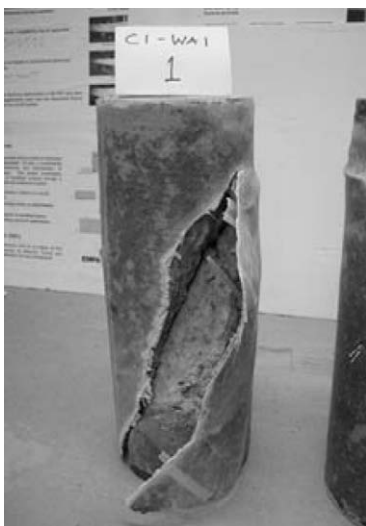
Fig. 3. Global shear cracking [2].
