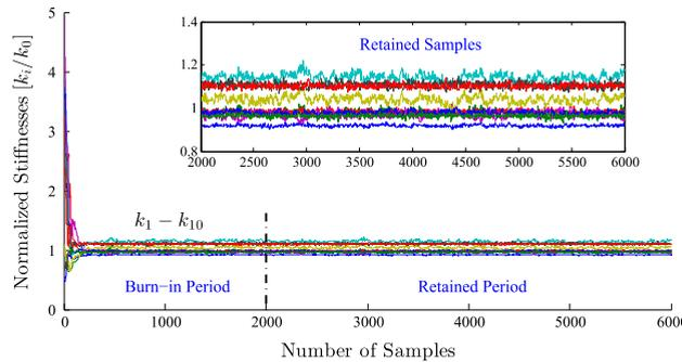
Fig. 2. Samples of 10 stiffness parameters of the 10-storey building obtained by MCMC using 20% RMS noise measurement.
