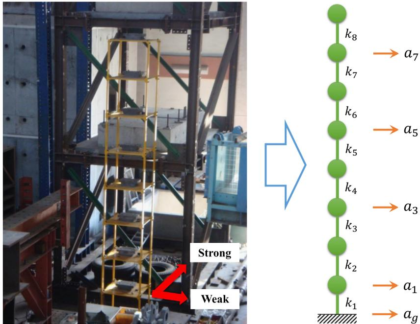
**Fig. 4.** Shaking table test setup of the 8-storey building. Note that measurements were recorded along the weak direction. The building is modeled by a 8DOF linear system.
