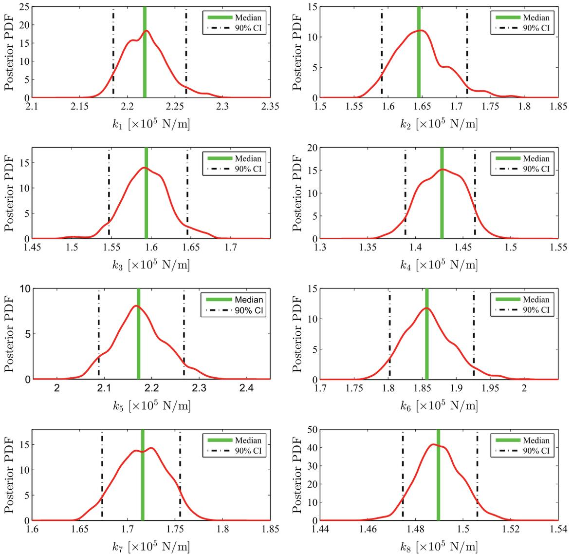
**Fig. 9.** The stiffness parameter posterior PDFs of the 8-storey building identified by MCMC using the shaking table test measurement. Note that CI represents the confidence interval.
