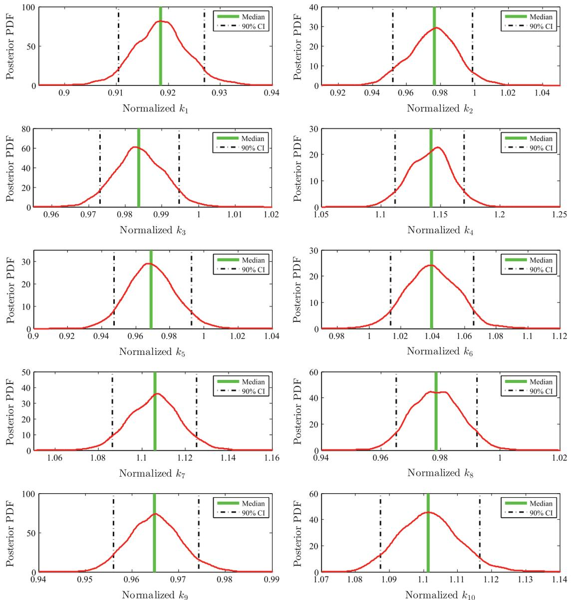
**Fig. 3.** The stiffness parameter posterior PDFs of the 10-storey building identified by MCMC using 20% RMS noise measurement. Note that CI represents the confidence interval.
