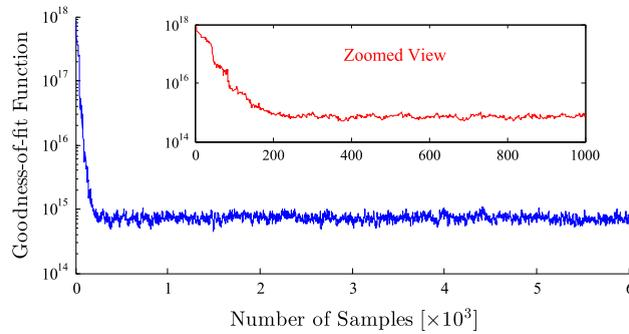
Fig. 1. Convergence of the goodness-of-fit function obtained by MCMC using 20% RMS noise measurement.
