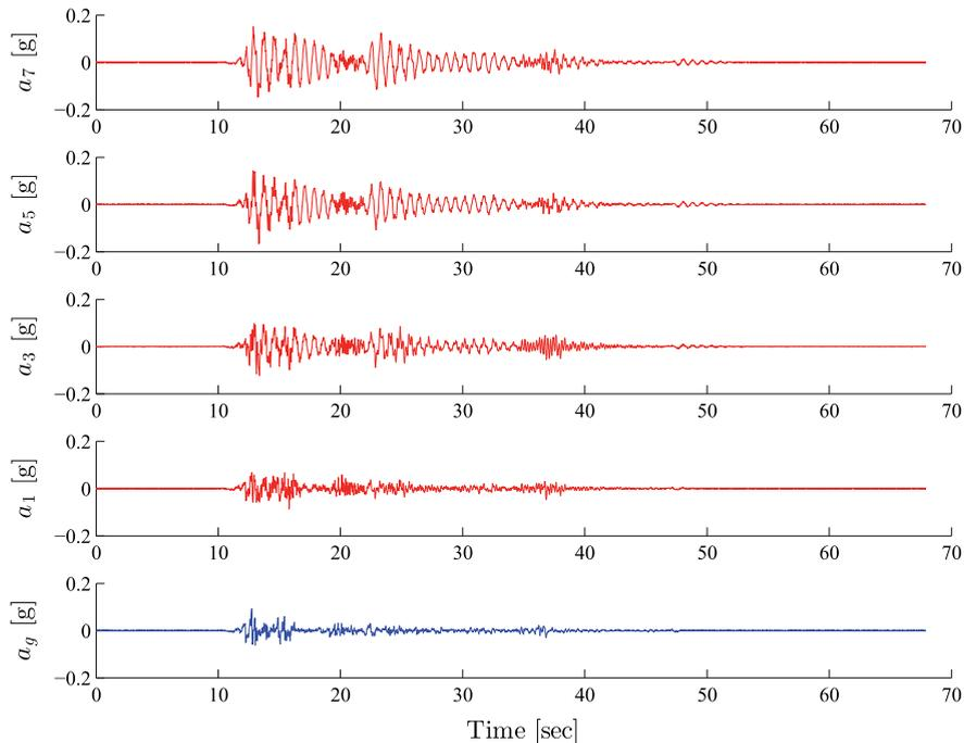
**Fig. 5.** A typical set of measured acceleration time histories of the 8-storey building.
