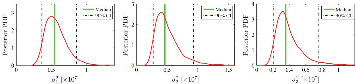
**Fig. 10.** The posterior PDFs of  $\sigma_1^2$ ,  $\sigma_2^2$  and  $\sigma_3^2$  sampled by MCMC using the shaking table test measurement. Note that CI represents the confidence interval.
