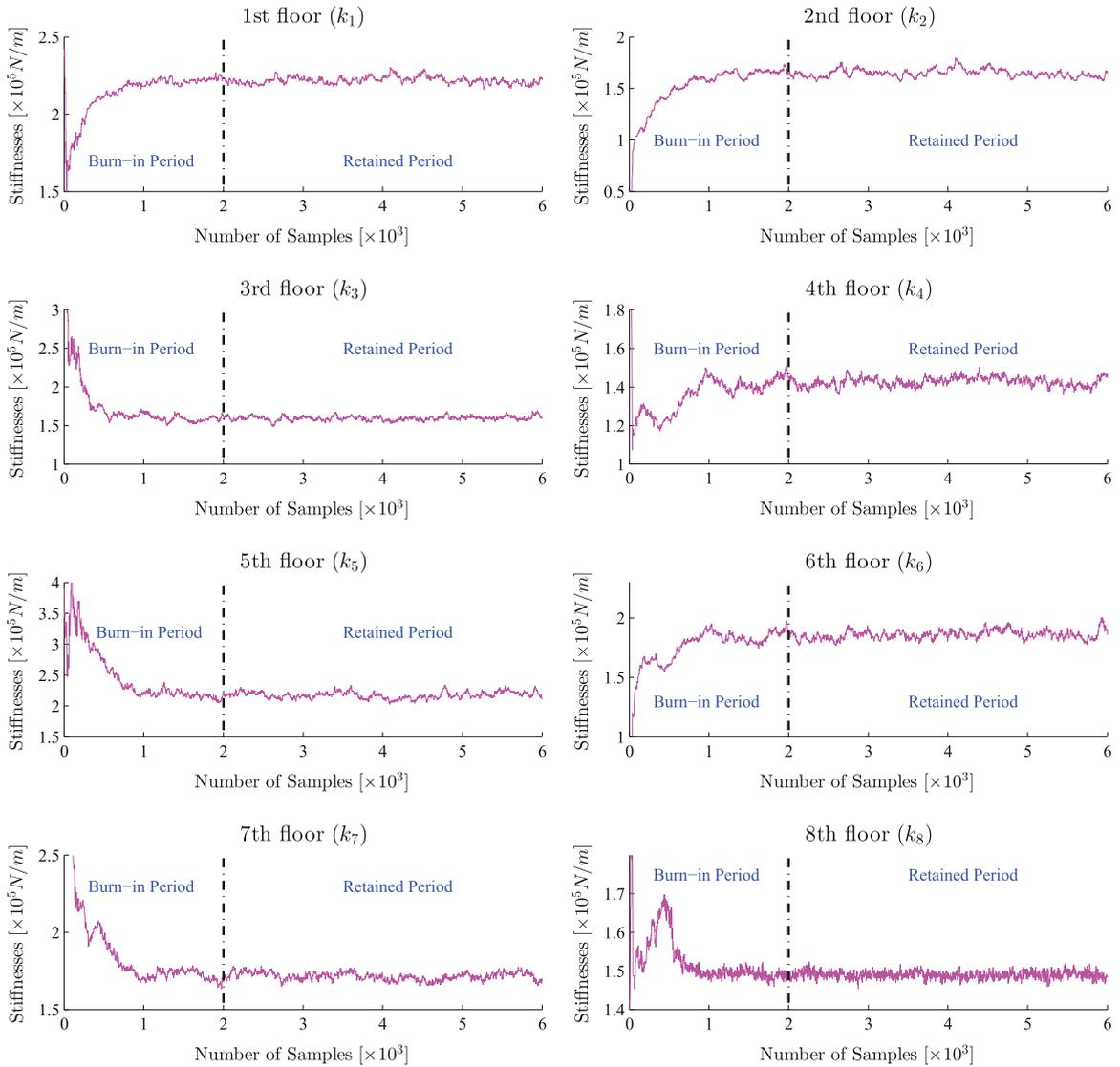
**Fig. 8.** Samples of eight stiffness parameters of the 8-storey building obtained by MCMC using the shaking table test measurement.
