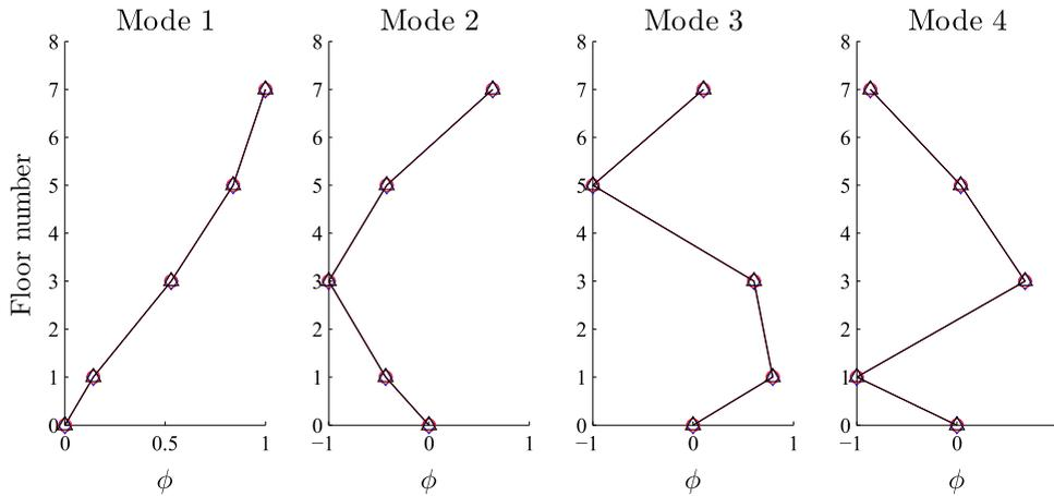
**Fig. 6.** Mode shapes of the 8-storey building identified by ERA-OKID using the shaking table test measurement. Note that the markers ( $\circ$ ,  $\Delta$ , and  $\diamond$ ) represent three data sets used herein.
