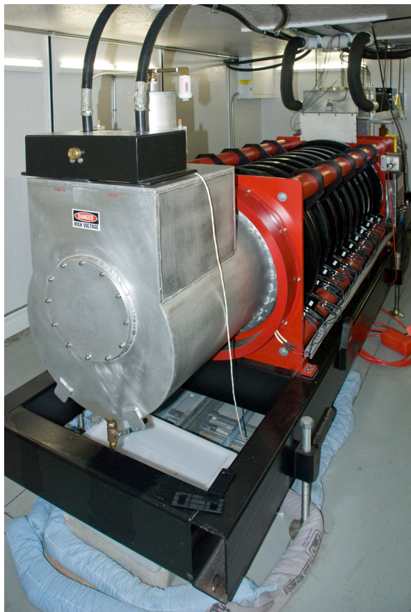
1 MW CW klystron 92kV at 17A 380 gpm of water
