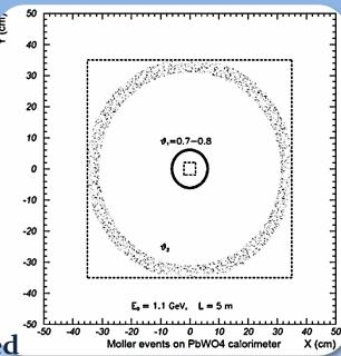
Double arm method: both Möller electrons are detected
