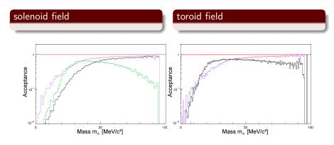
Blue: Reference from first estimations Black: Target in the middle of detector Green: Target at beginning of detector
