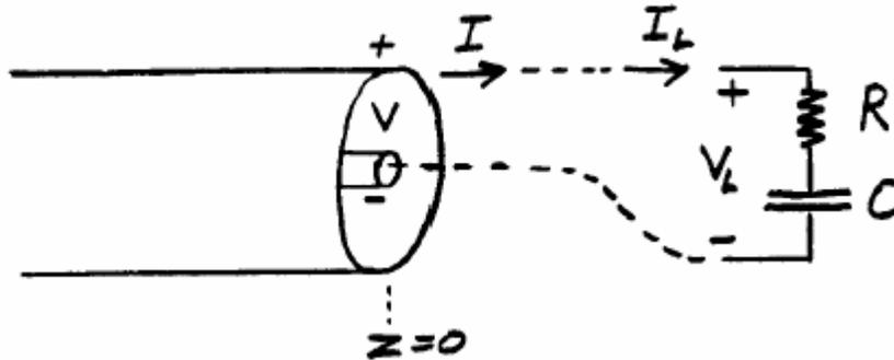
A coaxial cable with characteristic impedance  $Z_0$  is terminated by a series combination of a resistor and a capacitor as shown above. If a harmonic voltage wave is incident from the left, a reflected wave will be set up by the load. The resulting total voltage on the line will have the
