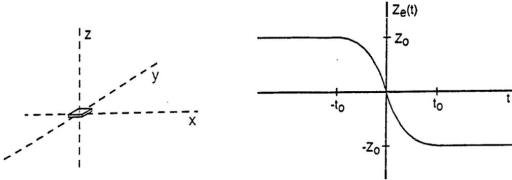
Avalanche breakdown in a semiconductor can cause a sudden motion of charge across a thin chip of material. In the example illustrated above, a small sample is located at  $\vec{r} = 0$ .  $N$  electrons of charge  $-|e|$  flow across a distance of  $2z_0$  in a time  $2t_0$ .
