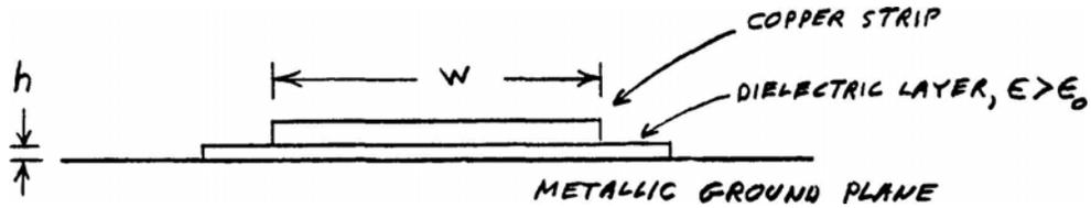
The diagram shows the cross-section of a microstrip transmission line that is used to conduct high frequency signals around circuit boards in many avionics applications.
