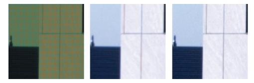
This shows the original Bayer pattern image, the result of demosaic\_linear(R), and the result of demosaic\_median(R). Median interpolation was performed by converting the result of demosaic\_linear(R) to YCbCr, filtering the chroma channels (Cb and Cr) with medfilt2, and reconstructing the luma channel (Y) using the original Bayer pattern image. The details of this technique will be covered in lecture.
