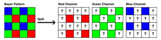
The above image shows the Bayer pattern for the provided PGM files (note that the top-left pixel is blue). Basically, your function should split the given image into three channels and fill in all the question marks in each channel. You may ignore the one-pixel border around the image. The PGM files are large, so you may wish to crop the images for testing.
