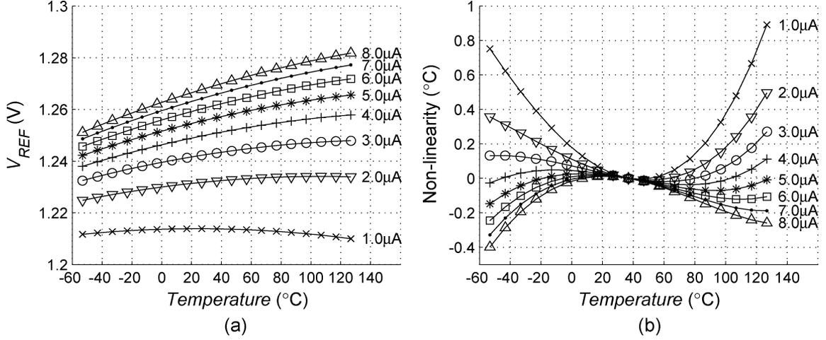
Fig. 3. (a) Simulated temperature dependency of the reference voltage  $V_{REF}$  as a function of the bias current at room temperature. (b) Associated nonlinearity of the sensor's output  $D_{out}$  (i.e., error with respect to a linear fit).
