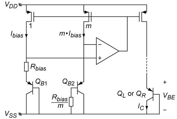
Fig. 9. PTAT bias circuit that makes  $V_{BE}$  independent of the forward current-gain.
