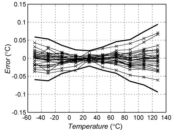
Fig. 16. Measured temperature error of 24 devices after trimming; bold lines indicate the average error and  $\pm 3\sigma$  values.
