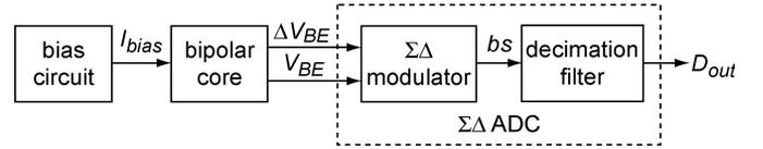
Fig. 4. Block diagram of the temperature sensor.
