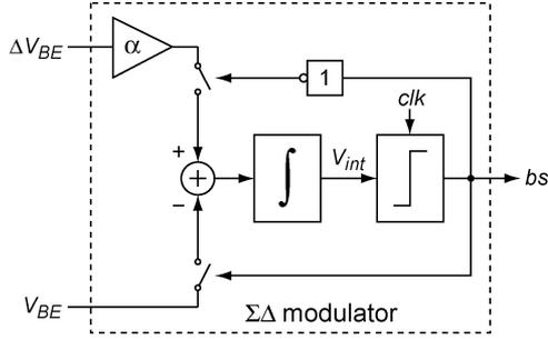
Fig. 5. Block diagram of the  $\Sigma\Delta$  modulator.
