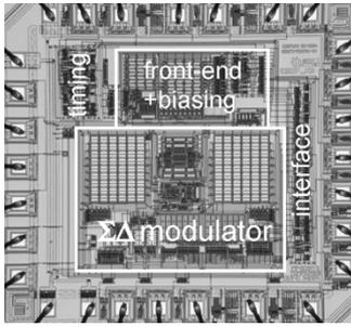
Fig. 13. Chip microphotograph of the temperature sensor.
