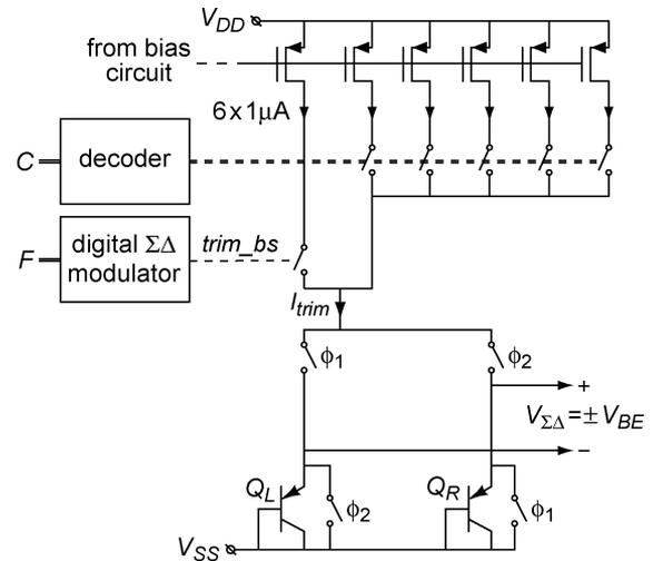
Fig. 8. Current-source configuration used to obtain a trimmable bias current  $I_{\text{trim}}$  for generating  $V_{BE}$ .
