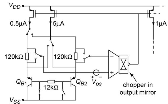
Fig. 10. Implementation of the bias circuit that uses chopping to cancel the offset  $V_{os}$ .
