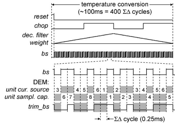
Fig. 12. Timing diagram of a complete temperature conversion.
