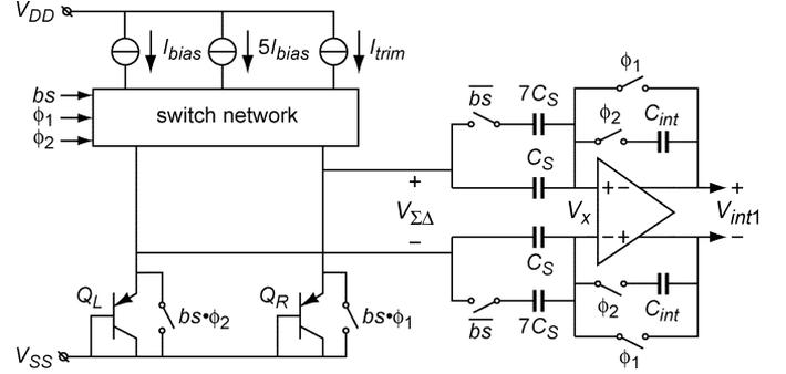
Fig. 6. Simplified circuit diagram of the front-end of the  $\Sigma\Delta$  modulator.
