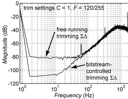
Fig. 14. Measured power spectrum of the bitstream, with the digital trimming  $\Sigma\Delta$  modulator operated in free-running and in bitstream-controlled mode (4096 bits,  $16\times$  averaged, Hanning windowed).
