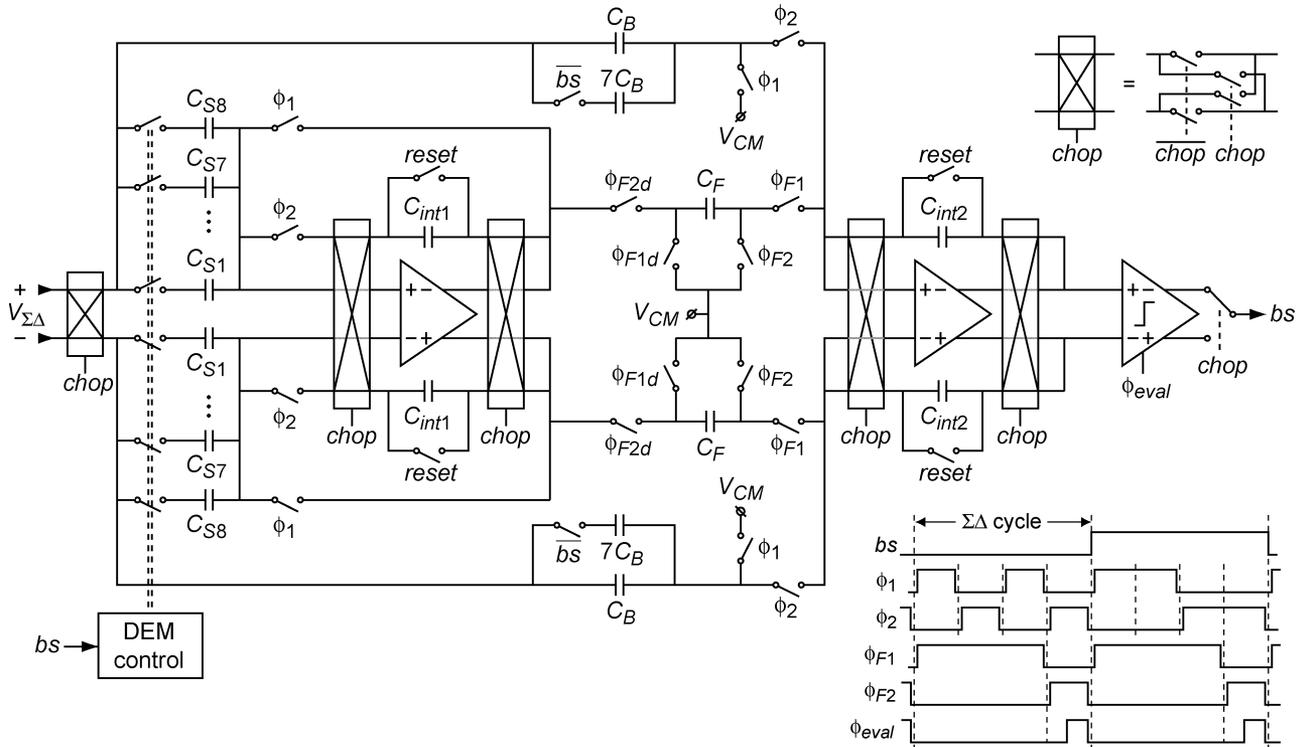
Fig. 11. Circuit diagram of the second-order  $\Sigma\Delta$  modulator.
