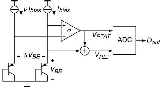
Fig. 1. Operating principle of the temperature sensor.
