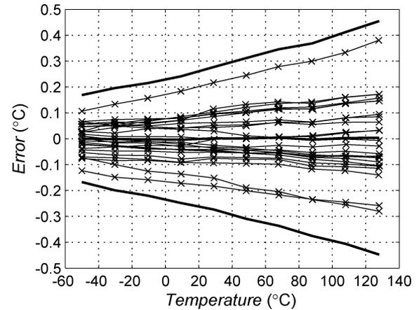
Fig. 15. Measured temperature error of 24 devices before trimming; bold lines indicate the average error and  $\pm 3\sigma$  values.
