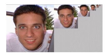
Figure 4-11: An image and its color mapping. The color mapping representation takes its input and downsamples it into a sequence of squares. Matching between images can then be performed by comparing the square representations of the two images being compared.
