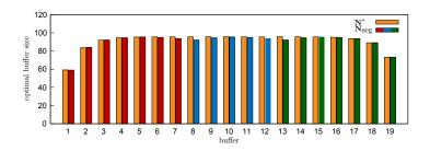
For comparison, we optimize the original 20-machine 19-buffer line directly and let  $\mathbf{N}^*$  be the optimal buffer distribution.
