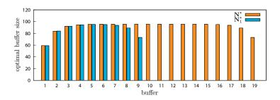
▶  $B_9$ ,  $B_8$ ,  $B_7$ , and  $B_6$  in the segmented line are reduced because of the zero variability downstream of  $M_{10}$ .
