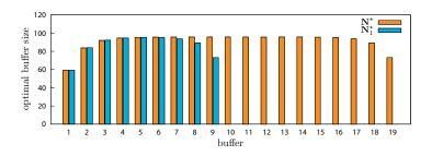
▶ B₁ to B₅ should be kept large enough to achieve the target production rate. This emphasizes the importance of the condition that the production rate constraint has to be active.
