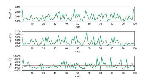
$r_i=.1$  and  $p_i=.01$ .  $b_i=c_i=1$ . The revenue coefficients A are 25,000 and 30,000 and  $\hat{P}=.88$  for both cases. 10-machine line segments are used in segmentation.
