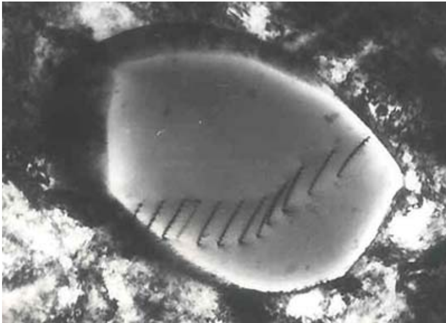
Transmission Electron Micrograph of dislocations (TEM)
