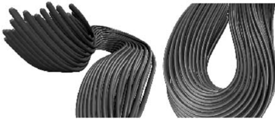
FIGURE 3.6 Simulation snapshot of response of a CNT bundle under mechanical compressive loading depicting significantly deformed/buckled shape. The bundle consists of 81 nanotubes using coarse-grain representation. (From Buehler, M.J., J. Mater. Res. 21(11), 2855–2869, 2006. With permission.)
