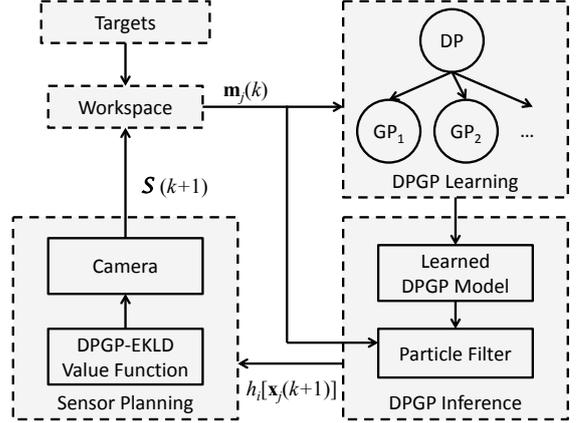
Fig. 1. Diagram of DPGP-EKLD sensor planning algorithms.
