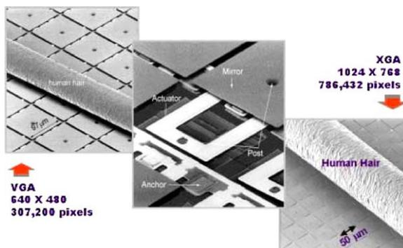
Fig. 2. Piezoelectric cantilever-actuated micromirrors for TMA display [3].
