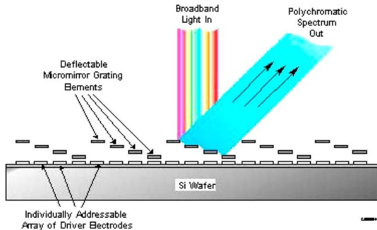
Fig. 4. Polychromator developed by MIT, Sandia and Honeywell [20].
