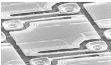
Fig. 5. Uncooled bolometer pixel (coplanar design by Honeywell) [21].
