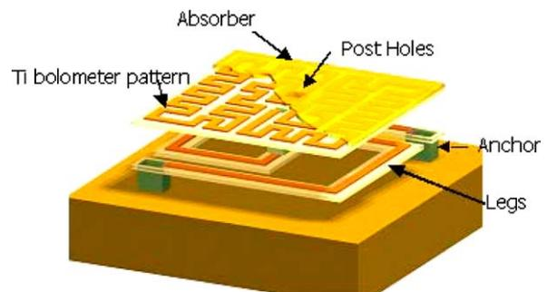
Fig. 6. Tri-level uncooled bolometer structure by Kim et al. [22].
