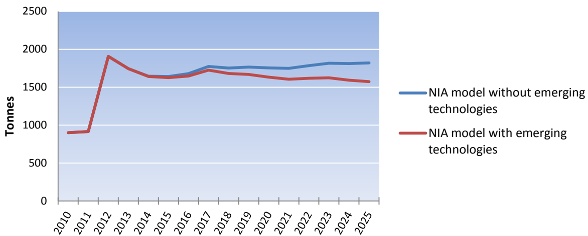
Figure 2-5. Comparison of Domestic Rare Earth Oxide Demand from LFL Phosphors under Different Assumptions for Emerging Technology Market Penetration
