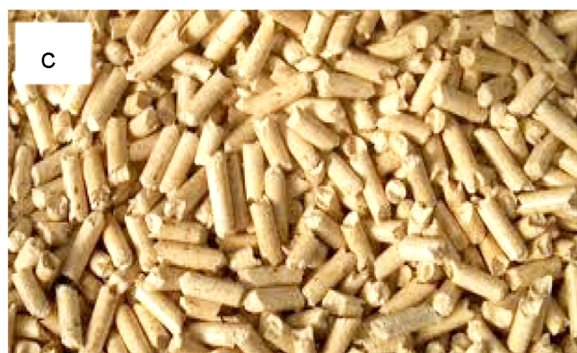
Fig. 1. Different forms of densified biomass: (a) bale, (b) briquette, and (c) pellet.
