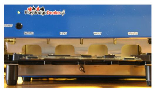
My Dealer4 with spring-loaded aluminum "flip plate" and navy blue "new generation" bridge board in place. The Dealer4 software requires the flip plate to be down, whether dealing into a board or onto the plastic plate. Poke a finger through a hole or tap the side of the board to clear leaning cards.
