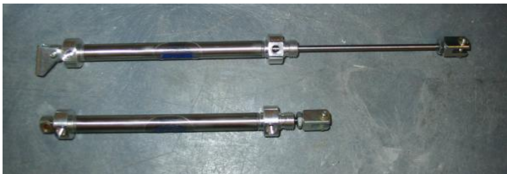
Figure 3-3: Pneumatic pistons used on grippers.
