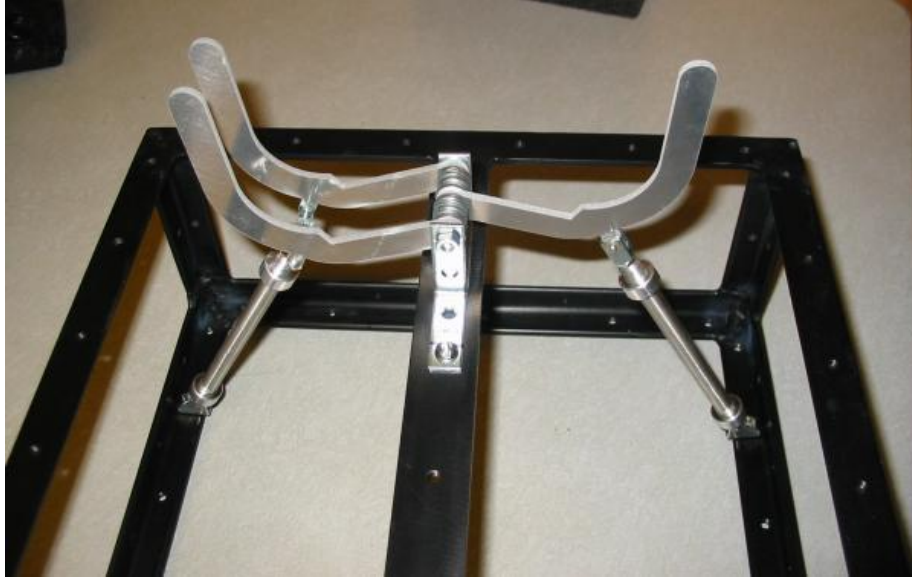
Figure 3-1: One pair of gripping jaws.
