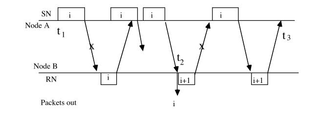
$t_1$  = time at which A first starts to transmit packet i
