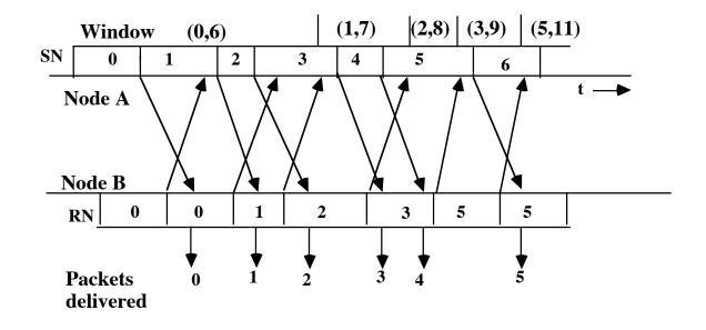
• Note that packet RN-1 must be accepted at B before a frame containing request RN can start transmission at B
