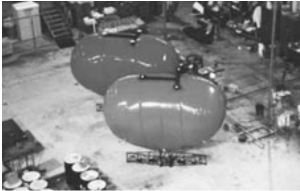
Figure 2 Stanford formation flight testbed using blimps
