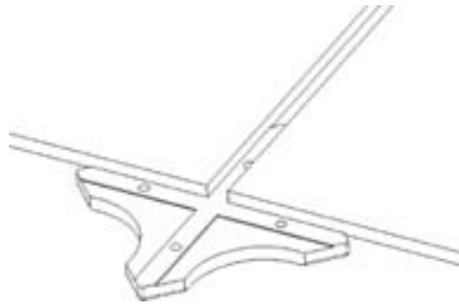
Figure 4. Depiction of bottom corner component with panel. The corresponding symmetrical corner component is not shown.
