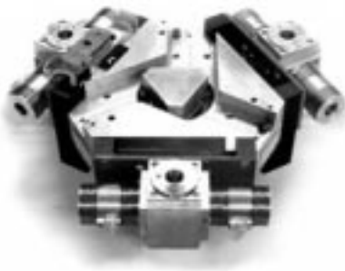
Photo: Prototype of HexFlex Nanomanipulator with magnet-coil actuators.
