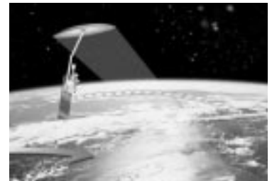
Graphic: Dara Entekhabi — The Hydros satellite will rotate to focus its beam for scanning a wide area of Earth's surface as it circles the planet every 90 minutes at an altitude of 670 kilometers.
