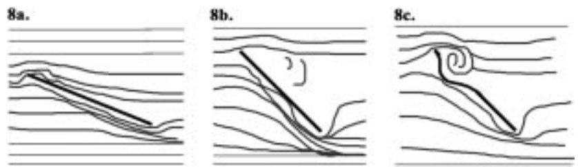
Figure 8. How angles of attack influence flow around an airfoil and how the fish may be preventing stall by passing a wave down the more dorsal fin rays. 8a: Relatively smooth flow at a low angle of attack. 8b: At high angles of attack, stall may occur if the leading-edge vortex becomes disconnected from the airfoil surface. 8c: By passing a wave from the fin ray bases to their tips, the fin may hold the leading-edge vortex to itself and thus prevent stall, allowing a continuous generation of thrust.
