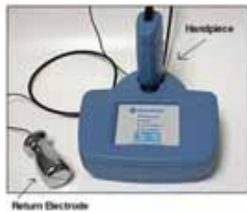
The SonoPrep device consists of a battery-operated power and control unit, a handpiece containing the ultrasonic horn and the disposable coupling medium cartridge, and a return electrode.
