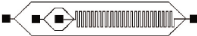
Figure 1. The schematic design of the microfluidic device.
