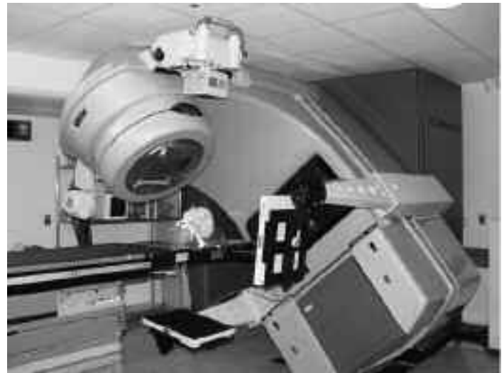
Figure 1. The IRIS system. Two X-ray imagers are mounted on the gantry of the Linear Accelerator and are orthogonal to each other.
