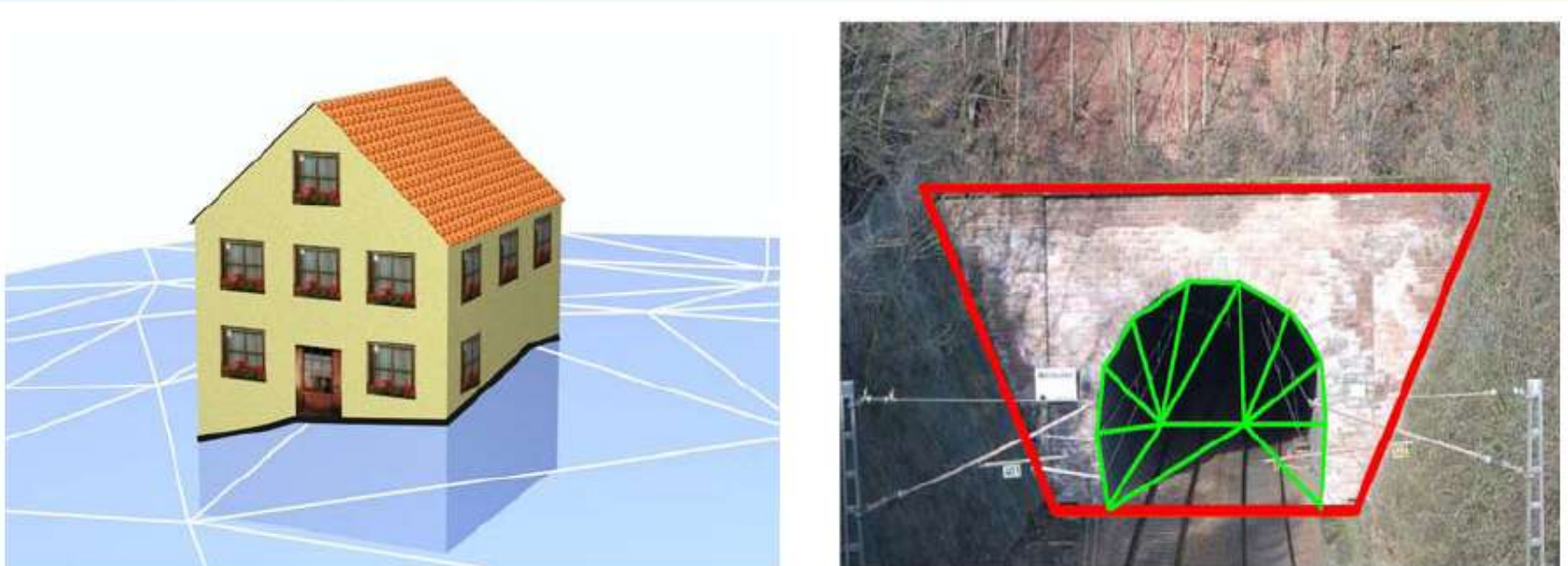
Fig. 5: TerrainIntersectionCurve for a building (left, black) and a tunnel object (right, white). The tunnel's hollow space is sealed by a triangulated ClosureSurface (graphic: IKG Uni Bonn).
