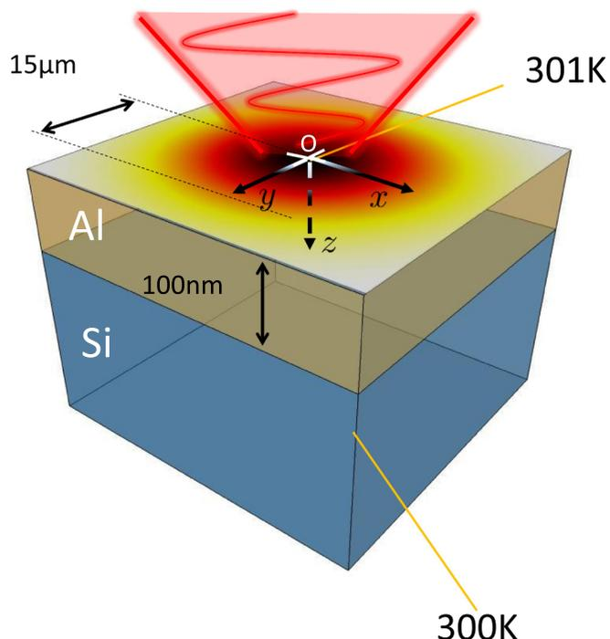
FIG. 1. (Color online) Schematic of a transient thermoreflectance experiment. Point O denotes the center of the heating pulse, also taken to be the origin of the Cartesian  $(x, y, z)$  set of axes. The system is assumed infinite in the  $z > 0$  direction and in the  $x$ - $y$  plane.
