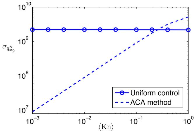
FIG. 9. (Color online) Standard deviation  $\sigma_{q_{x_2}}''$  of the particle contributions to the estimate of the heat flux at point A of Fig. 7 in the  $x_2$  direction, in the single free path model. In the ACA method, the standard deviation is proportional to  $\langle \text{Kn} \rangle$ . The latter outperforms the adjoint method with fixed control for  $\langle \text{Kn} \rangle \leq 0.2$ .
