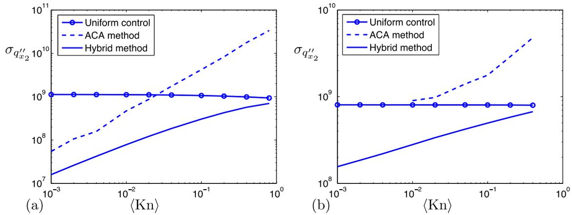
FIG. 10. (Color online) (a) Standard deviation  $\sigma_{q_{x_2}''}$  of the particle contributions to the estimate of the heat flux at point  $B$  of Fig. 7 in the  $x_2$  direction, in the variable free path model. (b) Standard deviation  $\sigma_{q_{x_2}''}$  of the particle contributions to the estimate of the heat flux at point  $A$  of Fig. 7 in the  $x_2$  direction, in the variable free path model.
