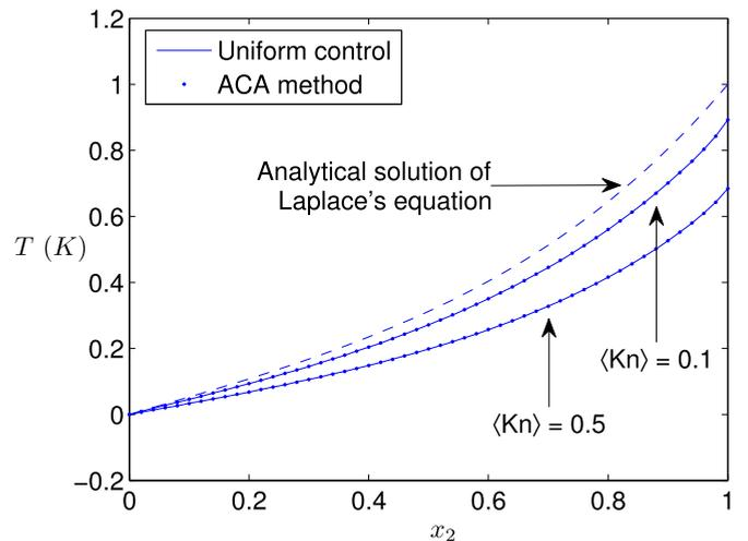
FIG. 8. (Color online) Temperature profile along the segment  $AB$  in Fig. 7. Comparison between the solution to the BTE calculated using the adjoint method of Sec. III A and the ACA method of Sec. VI A. The analytical solution of Laplace's equation is also shown.
