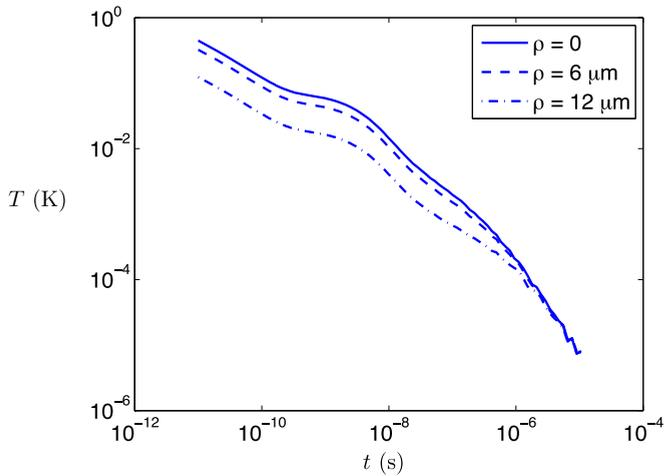
FIG. 2. (Color online) Temperature as a function of time in a transient thermoreflectance experiment. Results shown for the pulse center, 6  $\mu\text{m}$  away from the pulse center, and 12  $\mu\text{m}$  away from the pulse center.
