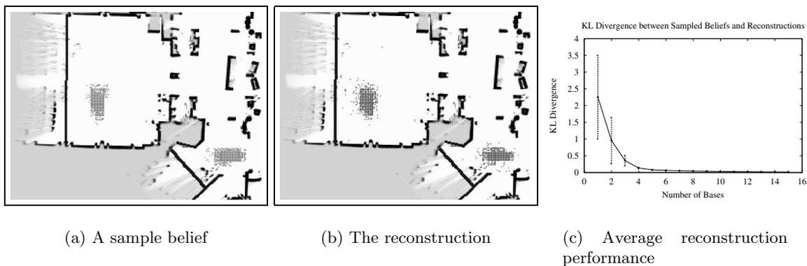
**Figure 13:** (a) A sample belief for the navigation problem in Longwood, cf. Figure 2. (b) The reconstruction from the learned E-PCA representation using 6 bases. (c) The average KL divergence between the sample beliefs and their reconstructions against the number of bases used.
