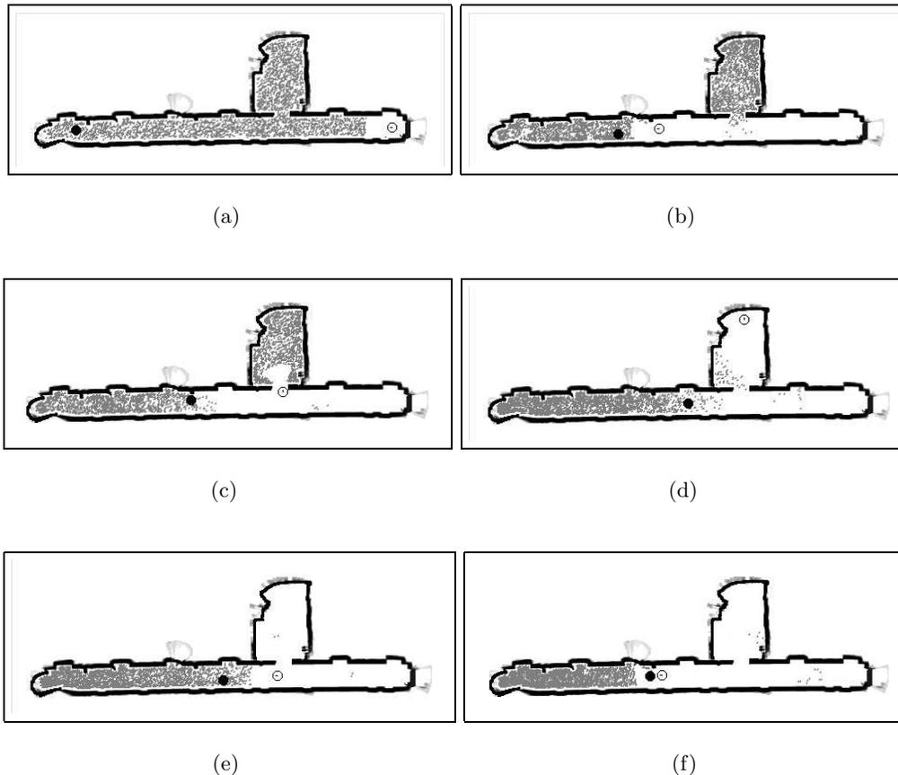
**Figure 21:** The policy computed using the E-PCA representation. The initial conditions in panel (a) are the same as in Figure 20. Notice that, unlike the previous figure, this strategy ensures that the probability mass is located in one place, allowing the robot to find the person with significantly higher probability.
