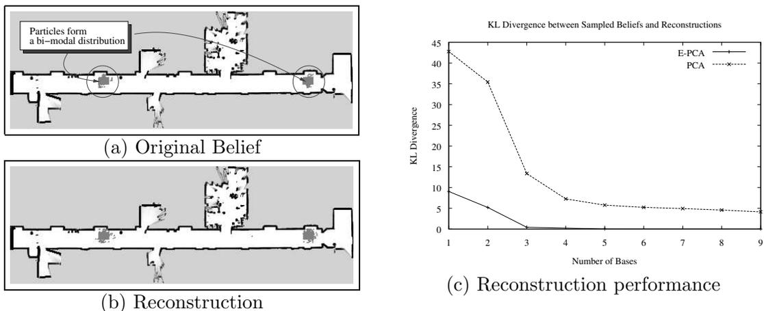
**Figure 12:** (a) A sample belief for the robot navigation task. (b) The reconstruction of this belief from the learned E-PCA representation using 5 bases. (c) The average KL divergence between the sample beliefs and their reconstructions against the number of bases used. Notice that the E-PCA error falls close to 0 for 5 bases, whereas conventional PCA has much worse reconstruction error even for 9 bases, and is not improving rapidly.
