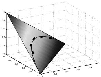
**Figure 6:** A one-dimensional surface (black line) embedded in a two-dimensional belief space (gray triangle). Each black dot represents a single belief probability distribution experienced by the controller. The beliefs all lie near the low-dimensional surface.
