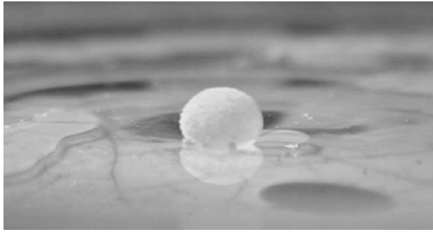
Fig. 9. Millimetric marble of water coated with a hydrophobic powder floating on water (courtesy Pascale Aussillous).
