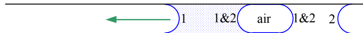
Figure 9: An air bubble as a spacer between the two miscible liquids slows down the mixing.
