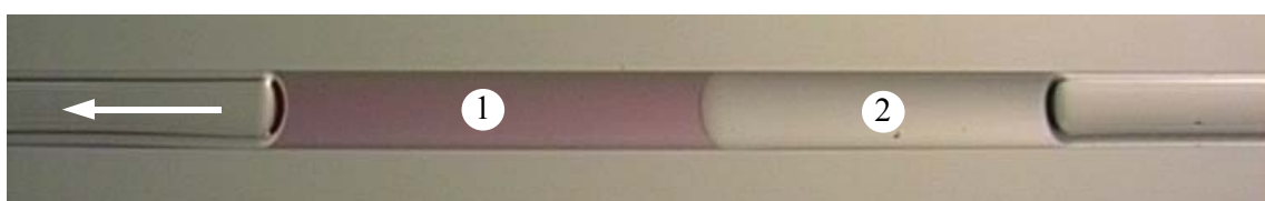
Figure 2. A bislug composed of two wetting liquids spontaneously moves in a tube. Here, the liquids are ethylene glycol and silicone oil, and they are juxtaposed in a glass capillary tube of millimetric diameter.
