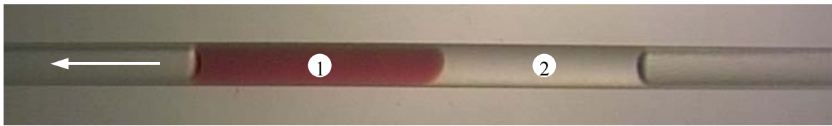
Figure 7. Inverted middle meniscus: ethanol /silicone oil bislug in a polyethylene tube.
